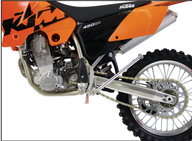
2004 KTM 450SX Kickstand Installed
