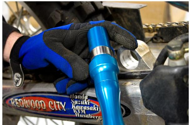
6. Place the new bearing onto the bearing extractor and then into the installation adapter with the recess facing the bearing. Then insert handle into Installation adapter as shown.
