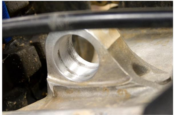
5. Carefully clean the inside of the swing arm bearing surface using fine scotch-brite and contact cleaner to remove any burrs or corrosion.
