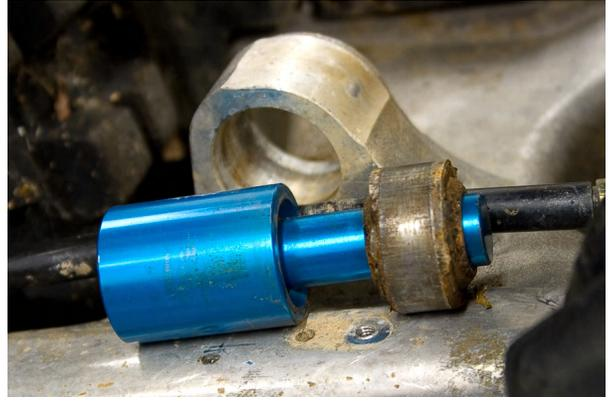
4. Place the bearing extractor on the handle and insert through the center of the heim joint. Drive the bearing out using a mallet.
