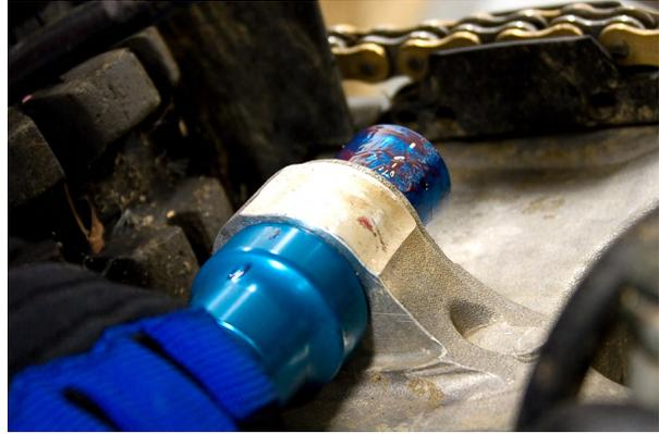
7. Place a light coat of grease or assembly lube on both the bearing and the bearing extractor to prevent damage during the installation. Rotate the flat portion of the installation adapter so it is aligned with the flat on the shock mount boss. Using a mallet, drive the bearing into the boss until it is fully seated against the installation adapter.
